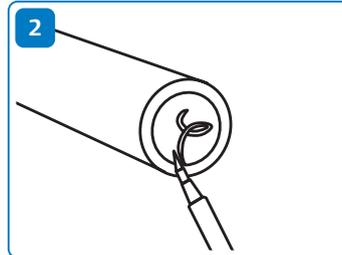
Bevel the pipe from the inside using a bevelling tool or a knife and remove possible bevels left outside the pipe.
