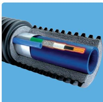
For liquids and water transport at extremely low temperatures, Uponor Supra Plus is supplied with a self-regulating freeze protection cable. It makes good sense to use this product if the pipeline is installed in conditions lacking weather protection, i.e. above ground or in shallow burial situations. The cable, rated at 10 w/m will prevent freezing down to  $-20^{\circ}\text{C}$ .
