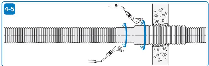
Place the shrink sleeve centrally in the joint between the sleeve pipe and the pipe element and remove any paper that may be left inside the shrink sleeve.
