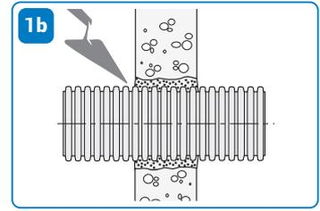
Place the feed-through sleeve in the structure where the pipe element will be placed and cast into place at a later stage. Please note that at least 10 cm of the sleeve pipe should be left outside the cast.
