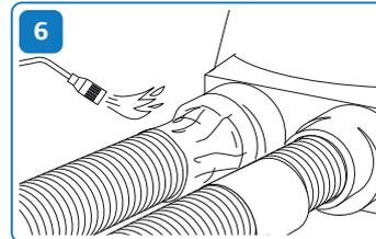
**6** Shrink it with a soft gas flame according to the instructions on the shrink sleeve. First shrink the end near the chamber, then shrink towards the pipe element. Keep the flame in constant movement.
