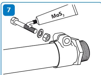
Tighten the WIPEX fittings. Lubricate the threads and washer of the bolt prior to tightening it. Use a suitable type of grease, such as silicone grease. Tighten the nut carefully using a spanner. Hold the bolt in place using a second spanner while tightening the bolt.
