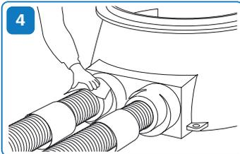
**4** Roughen up the surface of the jacket and the chamber joint with sand paper around the shrink sleeve. Wipe the joint area clean.
