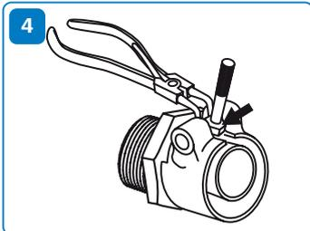
Place the bolt between the outer sleeve jaws and remove the outer sleeve.
