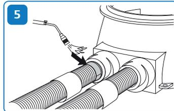
**5** Preheat the area that is left under the shrink sleeve using a soft gas flame. Remove the protective paper from the sleeve and place the sleeve around the joint.
