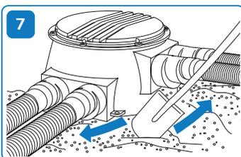
**7** Close the chamber lid, but tighten the bolts only after the pipeline has been pressure tested. Begin filling the trench by pushing sand underneath the joints.
