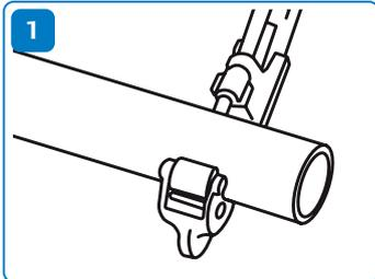
Cut the pipe at a right angle using a pipe cutter intended for plastic pipes.
