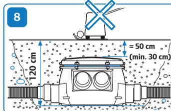
**8** Start the filling using a shovel, be careful not to damage the shrink sleeves. Check that the chamber stays upright. Compress the fill in layers of approximately 20-30cm. Mechanical compression directly above the chamber is forbidden.
