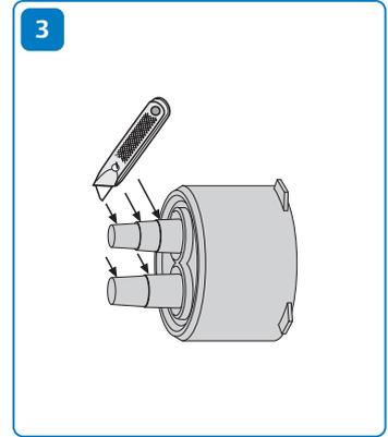
**3** Open outlets on the rubber end cap according to the flow pipe size.
