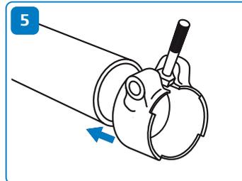
Push the outer sleeve over the pipe. **Please note!** Check that the outer sleeve has been turned in the correct position (the juts must be pointing towards the support sleeve). Installation of the pipe is easy and the o-ring remains undamaged when the o-ring is lubricated using a suitable lubricant (for example silicone spray).
