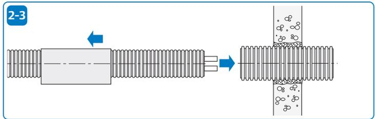
Install the shrink sleeve on top of the pipe element.
