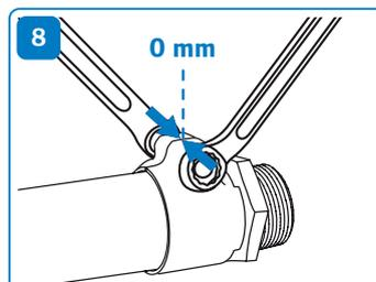
Tighten the outer sleeve so that its jaws touch. Tighten again carefully. If the jaws do not touch, wait for at least 30 minutes before re-tightening them.
