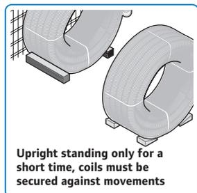
Upright standing only for a short time, coils must be secured against movements
