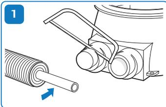
**1** Cut open branches of the chamber according to the required pipe size. Peel off enough of the jacket pipe and insulation to make the joint, 10-20 cm depending on the pipe size.
