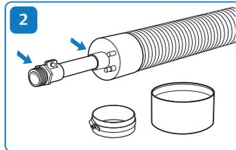
**2** Put the end caps and their seals in place at the ends of the pipes. Mount the connectors to the ends of the flow pipes. Slide the shrink sleeves onto the pipes.
