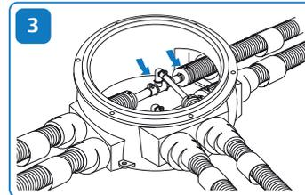
**3** Push the pipes into the chamber. Fasten the rubber end caps on the jacket pipe using jubilee clips. Join the pipes and tighten the couplings.
